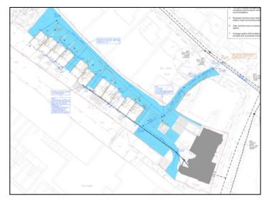
The additional intrusive investigations proved to be a successful and additional locations where suitable infiltration were identified onsite. GCA were then able to incorporate a design which utilised the permeable sub-base within the access road and car parking area for attenuation. This enabled the design proposals to be achieved without significant redesign, thus ensuring the scheme was delivered on time and within budget.
